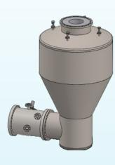
The burner is only used to preheat the system during the initial start-up phase or at times the media be temperature falls below the lower operating limit.
