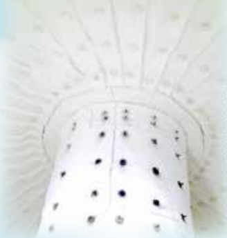
Figure 6 - Ceramic fiber blanket, dip tube and reactor walls
